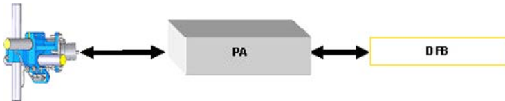
Fig. 4 Block diagram: the three analog signals are amplified by the preamplifier (PA) and then digitized by the digital field box (DFB)
