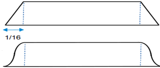
FIG. 20.2: trapezoidal apodization of the signal for the calibration of a spectrum
